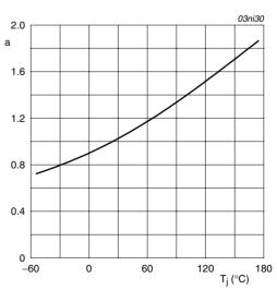
$a = \frac{R_{DSon}}{R_{DSon(2.5^{\circ}C)}}$
